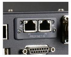
Fieldbus (Profinet or Ethernet/IP)
