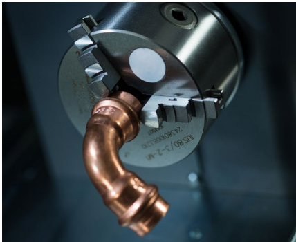
Rotary accessory for cylindrical parts marking
